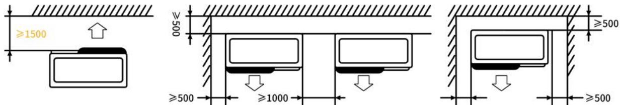
Do not put anything when the distance from the heat pump is less than 1 meter.
