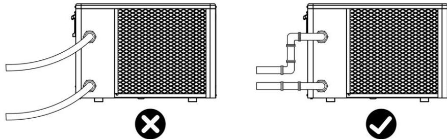
2. In order to guarantee the heating efficiency, the water pipe length should be  $\leq 10\text{m}$  between the pool and the heat pump.
